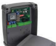
750D770M Electronic control unit for one or two 230 V gate operators with soft-stop and built-in 433,92 MHz rolling code radio receiver, complete with enclosure
