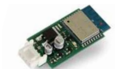
250T-WIFI Device for Wi-Fi connection 2,4 GHz to allow the smartphone to remotely control and program the control units via TauApp
