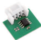
250SM126 Memory card for 126 radio codes
