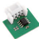
250SM254 Memory card for 254 radio codes
