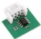
250SM254 Memory card for 254 radio codes
